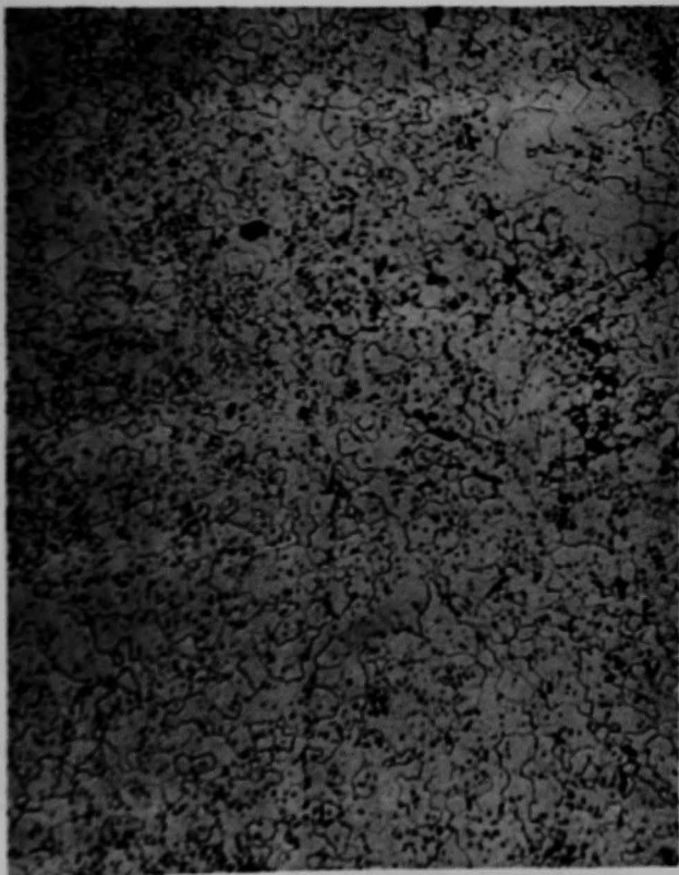
Figure D-52. Optical photomicrographs of particle 3 in the etched condition (typical).
