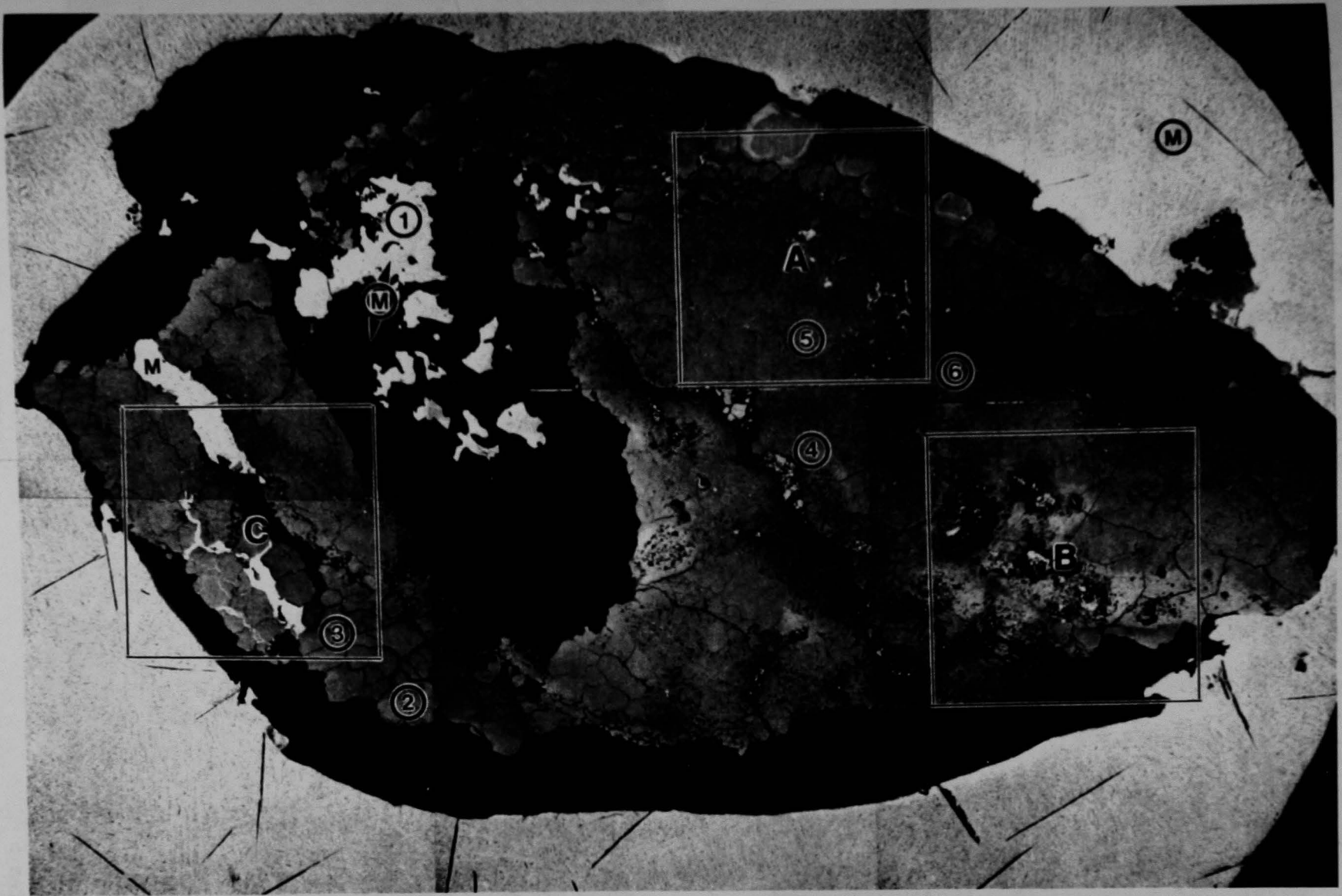
Figure D-23. BSE/SEM photo of particle 6. Areas 1 through 6 from Fig. D-21 are indicated. Areas A, B, and C were used for elemental dot maps.
